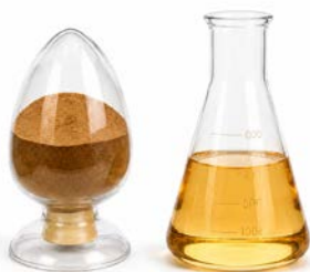
Naphthalene-based Superplasticizer (SNF)
